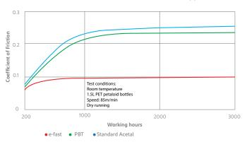
With the elimination of external lubricants, line cleaning is only required for sanitation. DuPont customized its Delrin® Renewable Attributed grade for e-F.A.S.T. material with a distinctive bright yellow color to help Regina's customers quickly identify the need for sanitizing.
